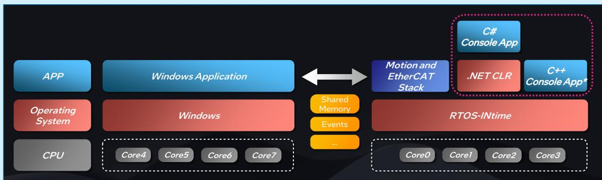
Figure 6. NoTime controller enables an application execution cycle of deterministic 125 microseconds<sup>5</sup>
