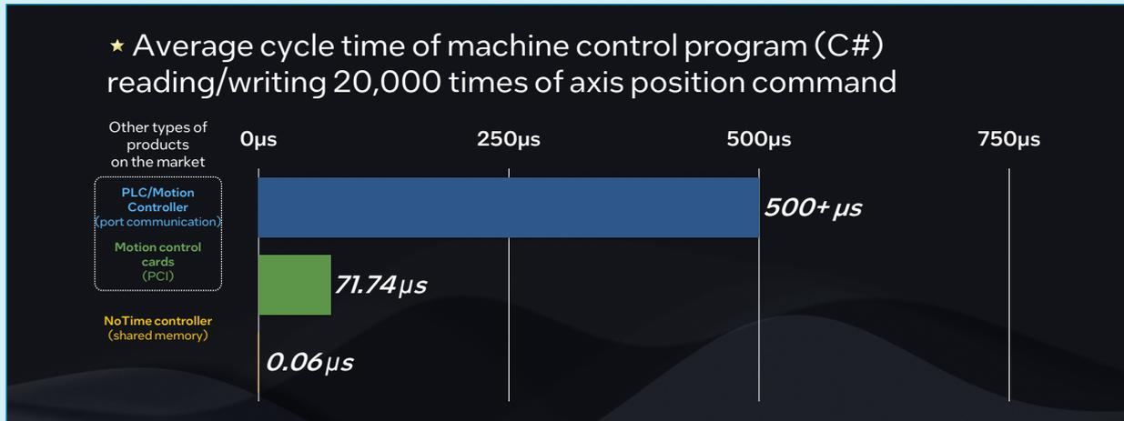
Figure 5. Time for machine control application (C#) to access motion control module (the lower, the better)
