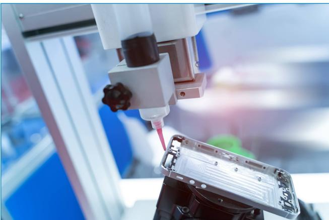
Figure 14. Dispensing process in cellphone manufacturing
