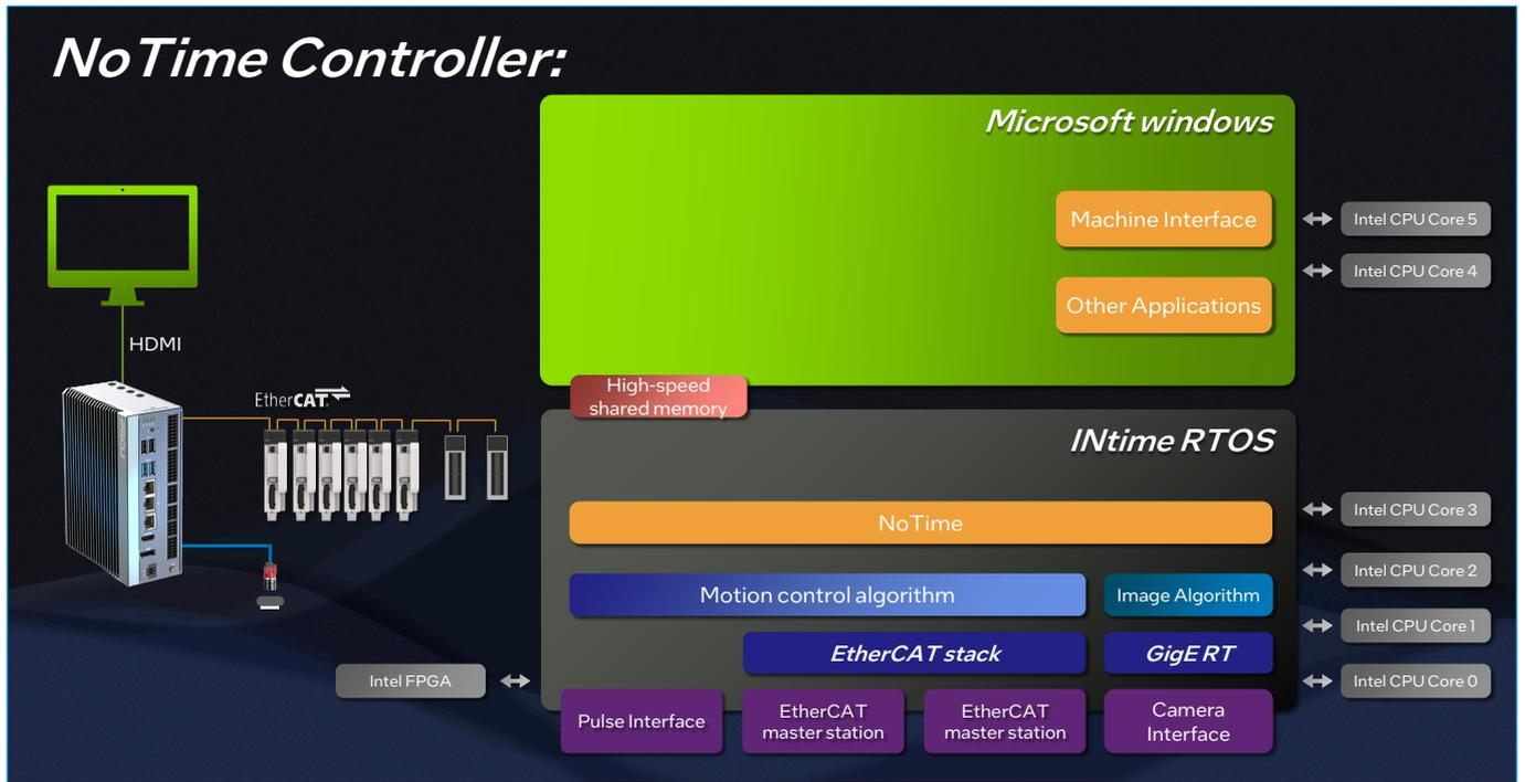
Figure 1. ProU NoTime controller design
