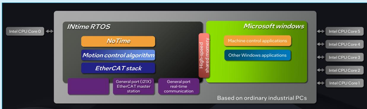
Figure 4. ProU NoTime controller integrates motion control application with machine vision software on the same hardware
