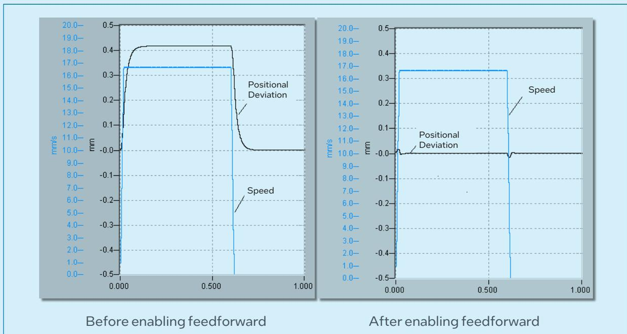
Figure 8. Comparison of position deviations before and after enabling feedforward control function
